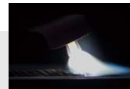
Triangular-wave TIG Welding
