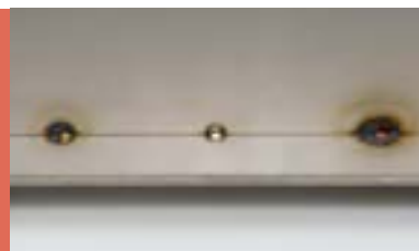
Spot welding function is not used
